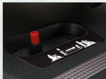
Two-step disengaging lever to prevent free-wheeling
